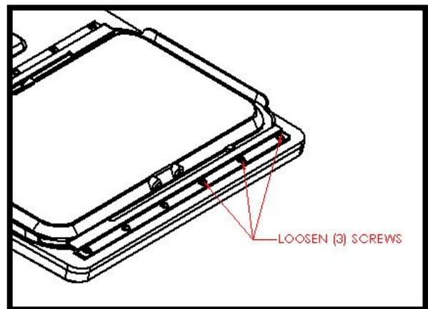
the rail slightly closer to the vanity and retighten the screws. Repeat the process with the other (3) screws on the same rail. If the vanity is too tight, use the same process but move the rail slightly farther away from the vanity.
